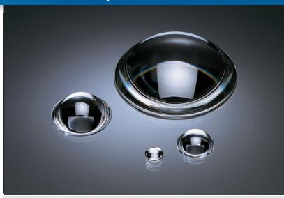
The lenses listed here have a molded aspheric surface as well as a second surface (R2) which is ground and polished. These lenses are mainly used in condenser or illumination applications. They are also used where a high light gathering power is needed such as for focusing onto detectors or fibers.
