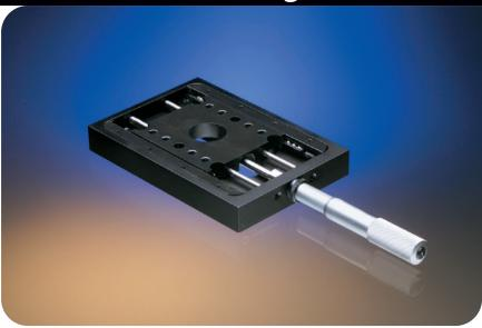
assembly. Spring-loaded guides maintain contact between translation stage and actuator driving head, ensuring an absence of 'stiction' and backlash.
