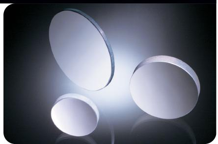
Ealing offers a range of protected aluminum flat mirrors in four different qualities. Select from interferometer to utility quality based upon the application at hand. The 25.4 and 50.8 mm mirrors can be held with our mirror mounts. The 76.2 and 101.6 mm mirrors would best be mounted with kinematic mirror mounts.
